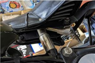
I also tried flashing the dynamo today to see if that would get it started. No joy so it will have to be a partial strip down to check the brushes and connections accessible whilst still on the bike.
