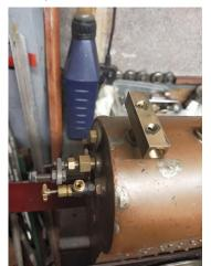
the items they will connect to. AS you can see, I do have the blower valve so I can make that up. A whistle valve is on order. The other two connection are for the injector (if I fit one) and the pressure gauge.
