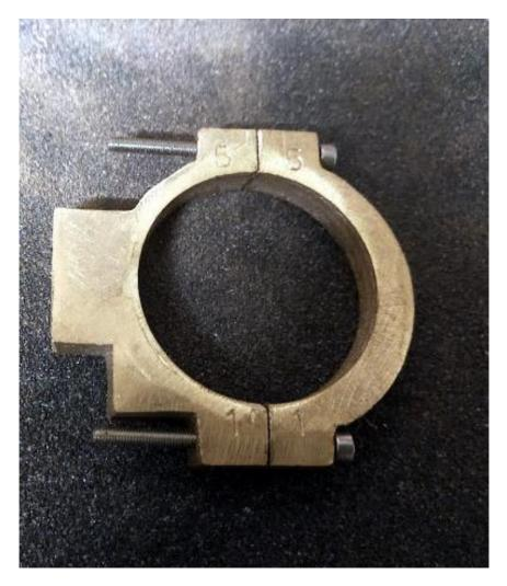
A little more progress with the water pump. I have fabricated the link between the eccentric strap and the pump plunger and this seems very satisfactory. As the picture shows the connector is presently bolted to the side of the eccentric. I am waiting for the mill to be installed to cut the slot.
