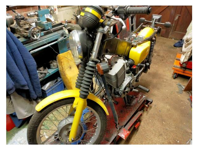
As you can see above I have fitted a drum brake wheel I had in stock for now so that at least I have a working brake. The disk brake assembly needs a lot of attention so has been parked for now. Last task today was to strip and examine the carb which was actually pretty clean. There was a twistgrip in the box of bits and this is now connected up. As we also have sparks, in theory the engine should run but not trying that just yet. This is meant to be a survey not the restortation.
