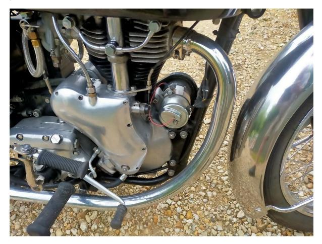
The wire by the way is because the body of the dynamo is painted and does not earth to the crankcase. It needs that earth to charge properly for some reason.
