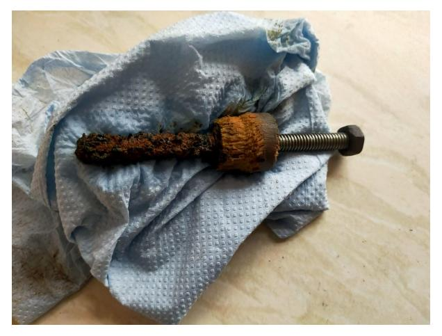
The picture above shows some of what came out of the oil tank , this was after the third iteration. The picture below shos the tank set up for electrolysis. For the oil tank I used the bikes 12v battery which worked ok but decided a bigger battery for the tank as it hold near 4 gallons of liquid.
