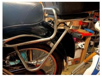
further investigation revealed that the two of the securing bolts for the rear mudguard had never been fitted. Of course it meant the wheel had to come out to get at them but they are now fitted and the carrier is finally secure.
