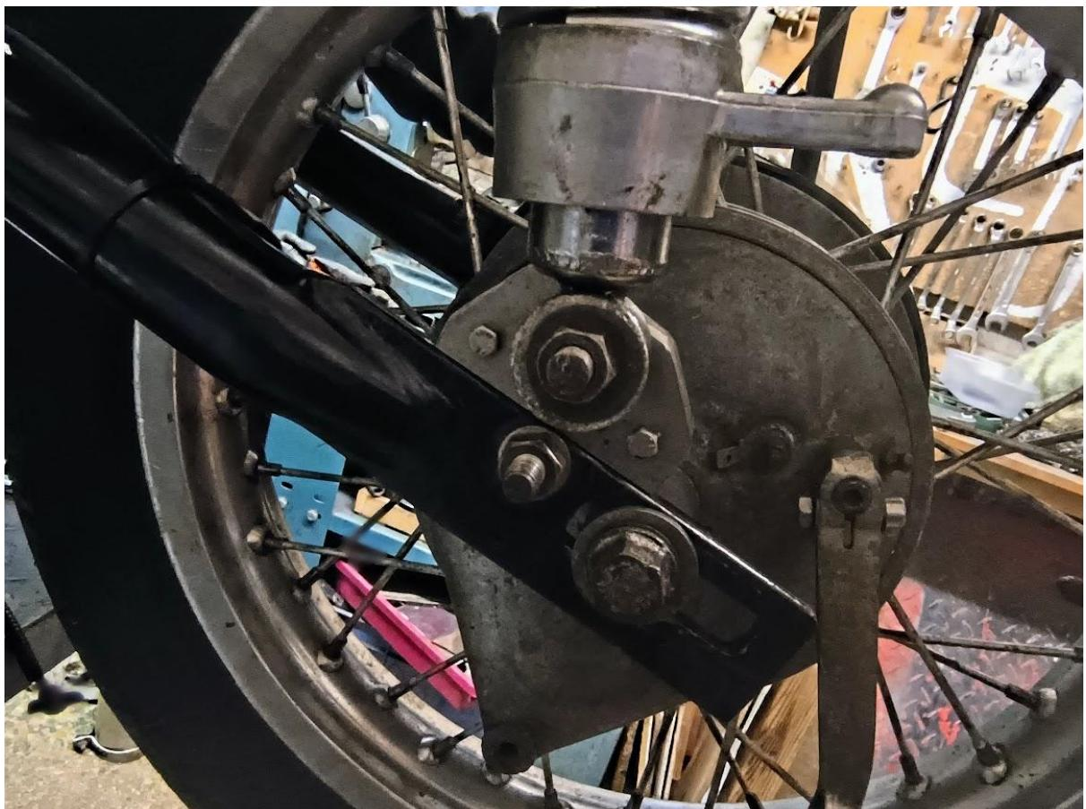
Its made of  $\frac{1}{4}$ " steel plate so should be plenty strong enough. This lifts the bike by 1" which will give clearance for an 18" rear wheel. The second picture shows the amount of clearance – though the 16" wheel is still fitted at present.
