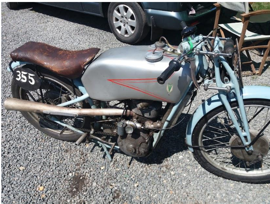
DKW 250cc 3 cylinder racer from mid 30's. Third cylinder is a compressor.
