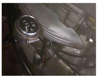
better job of attaching the pressure gauge so that I could ride the bike with it fitted on longer journey to get the oil really warm. Not elegant but it was the only place I could safely fit it and still be able to read it whilst riding along.
