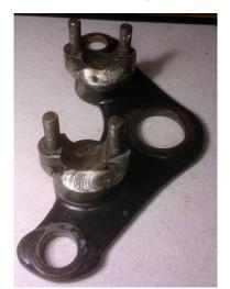
mounting for the handlebars. In fact the term should be reversion since with the paint removed it is clear to see that this is a genuine R26 yoke which has had clamps welded on afterwards, presumably
