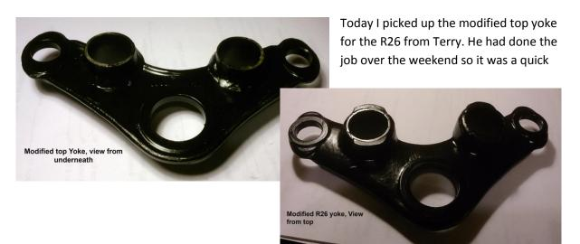
turn round. Back in the workshop I did some final tweaking to get the spacer tubes the right length and position in the bored out yoke, they were then taken to another friend (Mick) to be welded. He was a bit concerned about the composition of the metals and decided in the end to use nickel rods to avoid problems. Just as well I did not try to do the welding myself.
