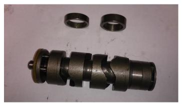
With rain stopping play I had another go at the Supa5 gearbox this afternoon and I may have identified the reason for the problems. The photo shows the selector drum and two spacers (called distance pieces in MZ speak). The thicker one (8.6mm) came from the suspect gearbox, the thinner (6.9mm) from another gear cluster. My suspicion is that the thicker spacer is a home-made item which in theory would help to push
