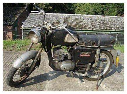
but I found a few that had not been done so gave those the treatment in the lather and polisher. The chrome cover for the rear light was not aligned properly so that was attended to as well. The stop light bulb is an LED as is the front parking light. Helpful with a 6v system though Ray has addressed a lot of the issues by fitting a relay to minimise voltage drop to the coil and a Velleman transistorized points gadget in place of the
