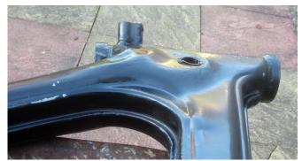
evidence of some trauma. However, things looked up when I offered up a journal bearing of the type used on all later MZS. It fitted the ETS stem perfectly and with a shim, would have fitted the frame. This was a pleasant surprise; what this means is that it may be possible to use the later TS150 frame as a replacement. I have the offer of one
