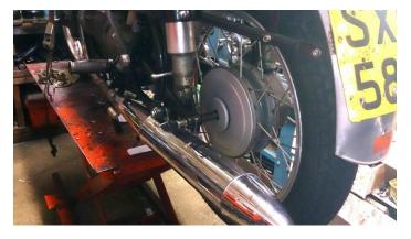
most of the repaired part is not readily visible so there is no immediate urgency about locating a better replacement. The back wheel now has s/s spokes and the ali rim is much shinier though not yet quite as a good as the front. While it was out I removed and painted the centre hub cap as well. I
