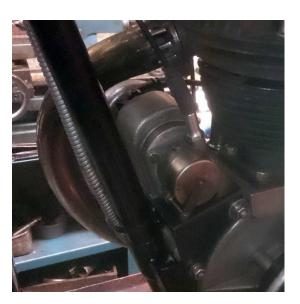
Apparently there should also be a guard to keep protect the mag so I am researching this to see if I can make one. I also need to repair the choke which fell apart the other day though the bike started easily enough with just a tickle. Bike will then go back into storage pending good clean & polish for the Bristol Show.
