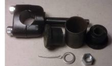
makes it clearer and my plan is to wholly remove the welded on bracket and bore out the yoke from the bottom to circa 26mm diameter to take the tube shown in the 3<sup>rd</sup> picture. This tube will retain the rubber bushes for the new handlebar clamps. Sadly most of this machining is beyond my skills and equipment so I am waiting for Terry to give me a date when he is free to do the job. In return I am going to fit a Powerdynamo kit to his Supa5.
