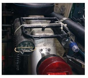
to the suspension top mount. I then made up a couple of brackets which are presently bolted
