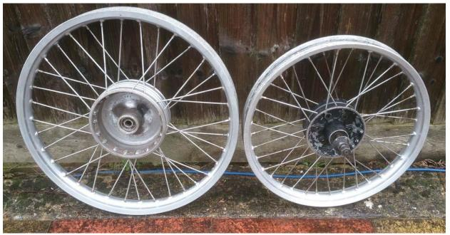
the front rim from the Trail TS150 and rebuilt the disk brake wheel as well. I don't have a particular need for such a wheel at present but it's more likely to be useful in this form than as a set of parts.
