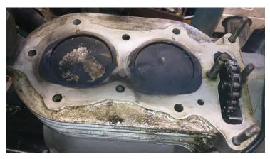
I only finished this today so no opportunity for a proper ride yet but the engine starts easily and seemed fine on a short ride round my test route. Part of the rebuild regime is frequent checks on the tightness of the head bolts so it will be a bit tedious for a while. Though there is no evidence of the gasket actually blowing, there does seem to be a suggestion of an oil weep from the head joint near the camshaft oil feed.
