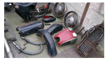
speedo are missing but both sets of brake linings are worn almost to the rivets so it is likely quite high. I have now sent a selection of the picture to Jim Lee and await his verdict. The obvious missing bits include headlight & speedo, both toolbox covers, the mudguard tail piece and rear light (and of course
