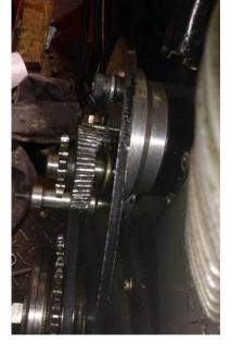
It could be bad assembly, poor maintenance or it could be a design fault. The fitting instructions sent by Alton show an outrigger plate that supports the spindle. However, this support plate requires certain other fixtures not present on my starter kit. I have seen a picture of the kit when originally fitted to my MAC and indeed there is no support plate. My guess is that Alton realised this was a weakness and modified later models.
