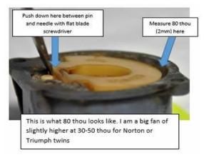
very low and the needle barely allowed any fuel to pass. But this does create an enigma; a low fuel level and flow rate would certainly cause misfiring but would surely also cause a weak mixture. Yet the plugs always showed signs of excessive richness. So far no one has come up with a plausible explanation for this phenomenon. I have run out of time to devote to the Venom for now, but when I get back from Spain I may decide to adjust the Wassell and have one more try at getting it to work.
