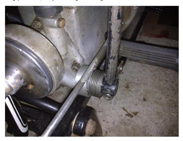
I also removed and had powder coated the footrests and rear brake lever as these were rusty and spoiled the look of the bike. These bits came back a couple of days ago and have now been fitted. Spurred on by this success I finally plucked up courage to take the bike out for a ride today. Apart from a binding back brake caused by forgetting to adjust it after fitting the footrest and brake lever, the bike ran well and we did about 15 steady miles mostly at 30-35 with an occasional burst up to 40.
