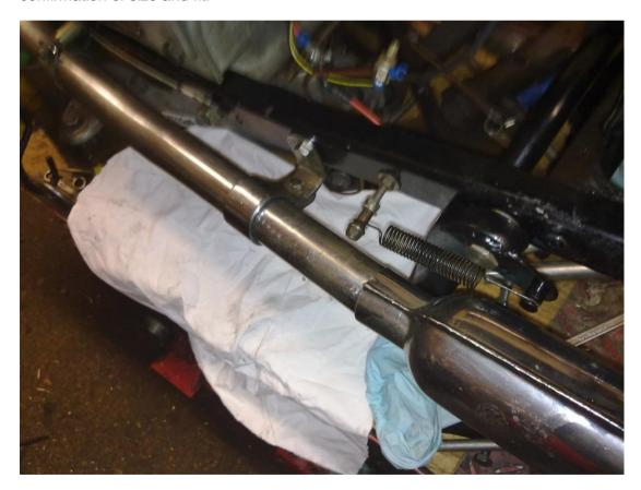
I then had ago at fitting the tank for the first time. The riders seat has to be removed first as the back of the tank will not quite slide under the front end of the seat. The front fixing bolt is very awkward to reach so I fitted a locked stud which the tank now drops on to and can be bolted up from the top. Fortunately, the back two fixings are easy to reach with ordinary bolts but rubber washers will be needed eventually. The
