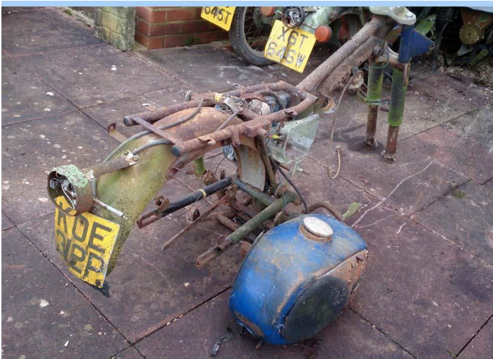
AUY886M - 1974 TS250 (4spd). On DVLA computer, The offside pillion tube has been cut off for some reason. It could be repaired by using one of the other frames as donor. The frame itself is otherwise in slightly better condition than the other 74 TS250 and it also would be tax exempt.
