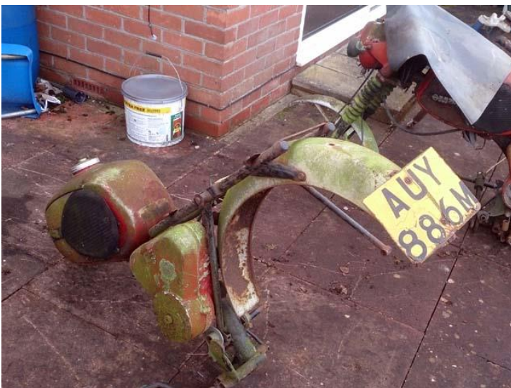
AUY886M - 1974 TS250 (4spd). On DVLA computer, The offside pillion tube has been cut off for some reason. It could be repaired by using one of the other frames as donor. The frame itself is otherwise in slightly better condition than the other 74 TS250 and it also would be tax exempt.
