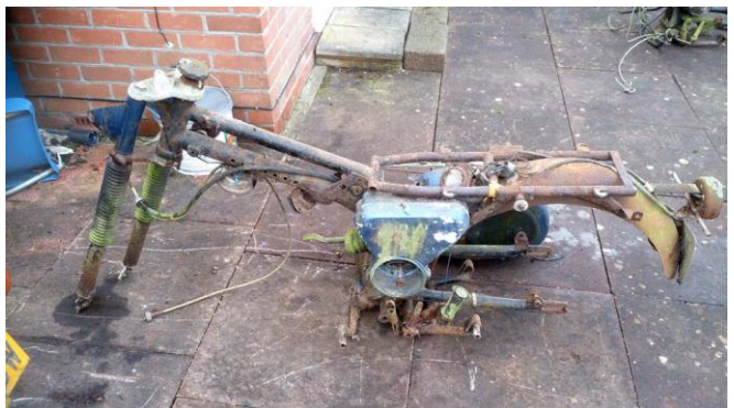
AUY886M - 1974 TS250 (4spd). On DVLA computer, The offside pillion tube has been cut off for some reason. It could be repaired by using one of the other frames as donor. The frame itself is otherwise in slightly better condition than the other 74 TS250 and it also would be tax exempt.
