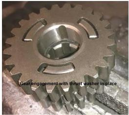
My next move was to very gently grind the outer circumference of the thrust washer such that it would fit inside the 1/3 slider gear recess. I then reassembled the cluster and now have gears which will fully engage with a little slack to allow them to move comfortably into position. I had already slimmed down the distance spacer to 7mm, in hindsight I wish I had left it a little wider as with my thrust washer alteration, it could safely be at least 7.5mm.
