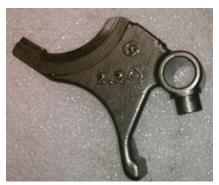
than measureable. It was far from the point where it was blackened from excess heat and half its original thickness which is how they normally appear once the gear jumping problems become starts. The selector drum
