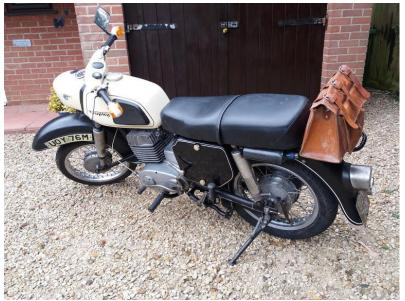
Putting stuff away in the loft the other day I noticed a sturdy leather bag and it seemed an ideal shape and size to fit on the Trophy. I found some old tubing which has been bent into shape with legs that slide inside the rear frame tube. Quite pleased with the overall result. Neater than a top box and ideal for carrying odd items of shopping.
