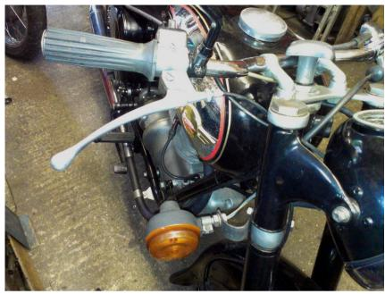
have a nice working set of front indicators. Still have not figured out a satisfactory mounting for the rear indicators and I will of course have to lay in extra cables. Put this on the back burner for now.
