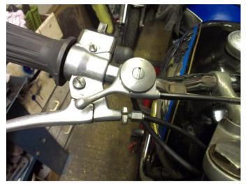
to dismantle the whole assembly and re-route the cable and while I was at it I fitted the Concentric choke assembly since it was now clear that the bike was very sensitive to weak mixture and needed better enrichment when cold. I had not bothered previously as the original BVF carb did not feature a choke, just a tickler. Finding a suitable choke cable took a while but eventually it was all back together and we finally had a result. The bike starts easily and revs from cold provided it has
