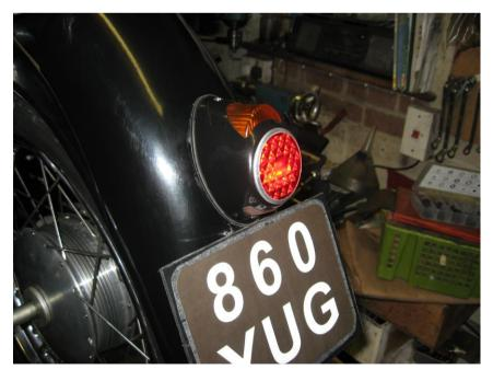
Fitting the actual light unit was fairly easy and I did not need to drill any new holes. In fact I was able to block up some spare holes with rubber grommets. Quite pleased with the overall result: Makes the number plate look scruffy so I will have to order a pressed aluminium one some time soon. They have gone up a lot recently near £28 now but they do look good.
