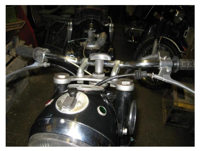
While I was working in that area I also made up a new clutch cable from an old but excellent condition BMW clutch cable. This is heavier gauge and nylon lined so should be quite smooth and light. Certainly far better than the old one which needed pliers to move the inner. I will send the old one to Venhill at some point to get a proper one made up to keep as a spare.
