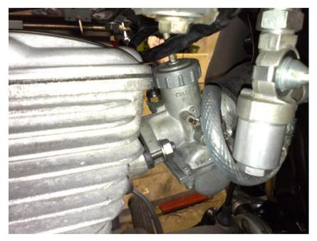
that the original carb only had a 105 jet). I then removed the slide and filed the base to reduce the cutaway. This also improved matters in the garage but on the road it was necessary to nurse the throttle and let the revs build up slowly. Rapid throttle action still made the engine die. I have the battered remains of a genuine VM24 carb so I compared the needles. The genuine needle was much slimmer so this was duly
