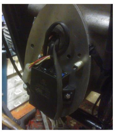
piece of rod internally threaded 6mm. This now screws down to a 6mm dowel in the crankcase and holds the plate firmly in position. I shortened the out fixing screw which now goes into the 20mm threaded rod. The picture probably makes more sense than the description.
