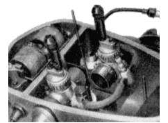
the other was about 4 turns out. Both are now et to 2 ½ turns out also per the manual. The throttle slide arrangement is quite unique and not just because of the flat slides. The slide is actually operated by a rod which terminates in a special housing which also locates the throttle cable. This complex arrangement is needed to allow the top cover to be removed and replaced easily. There are also buttons built into the top cover to
