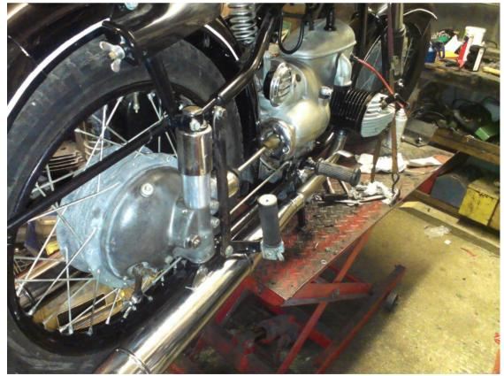
was simply impossible to get the system to align properly. I had more success with the near side and found a combination of pipe and silencer which aligned pretty well spot on. Out of interest, I tried the original off-side exhaust pipe with a new silencer and still no joy, the
