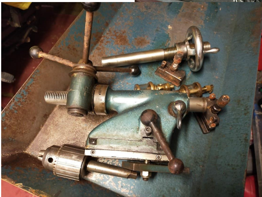
Tailstock, oilers and spare quick change tool holders as they arrived. The tailstock adjuster is an after-market quick action type. The original adjuster is at the top of the picture.
