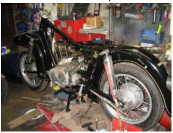
bit worried about clearance for the exhaust system. Fitting the rear mudguard and rear wheel was simple enough, though I found that I had overlooked painting the rear torque arm so this will have to be done later. With the wheel in place I was also able to fit the rear brake pedal and line up the rest of the brake connections. Final iob of the day was to fit the airbox, which also provides the mounting for the coil, regulator and fuse box. So
