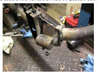
straight struts were relatively simple, The front one mated to a 40mm clamp on the front down tube. I was fortunate to have one of these already in the garage.
