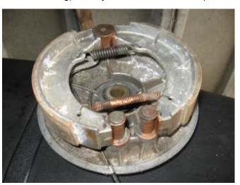
fitting the brake back-plate, I noticed that someone had modified the brake shoes. They normally pivot on pins at the back but these had been filed flat so that they can slide on the pins. In theory this should enable them to self-centre and keep maximum contact on the drum. Will be interesting to see how they perform.
