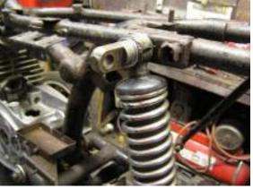
butted against the bottom engine mounting bracket so this made alignment easy and plenty of contact for welding. I was concerned about the small contact area at the front so added a metal loop having first checked it would not foul the engine. Surplus metal was then cut of with the angle grinder. The final result can be seen below.
