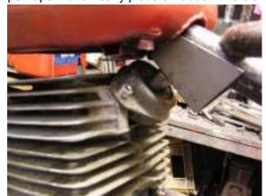
probably work, in a sense the later engines only have a single front mounting and can be seen jumping around particularly at tickover. I may yet have to fall back to this option. The second option was to fabricate and weld to the frame a top mount to hold the standard doughnut. This is an attractive idea; it would permit unlimited choice of engines from the later MZ range (a 301 would be nice). I successfully manufactured such a mounting after a few false starts, though I only clamped it to the
